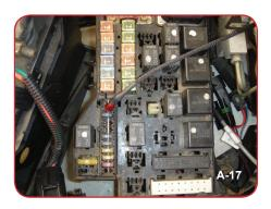
Now route the longer, red with a white tracer, power wire to the interior fuse panel. You may go through the same hole or slit you made to route the Control POD plug and wiring to the Adrenaline module for this power wire. Finally, attach the fuse tap to the leg of the #9 mini fuse (this is a 10 amp fuse) (Image A-18)
